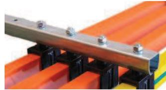
Assemble the supporting points for the conductor rail according to the specified distance (See page 5): every 1.500 mm. for profiles UP-1 and every 1.800 mm. for profiles UP-2.
