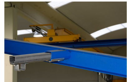
BEAM WELDED SUPPORT
