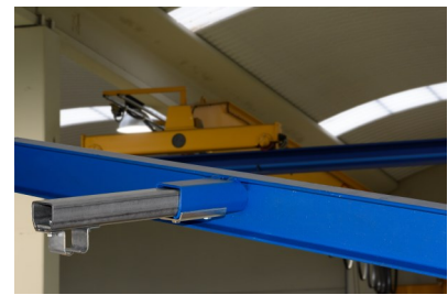
BEAM WELDED SUPPORT
